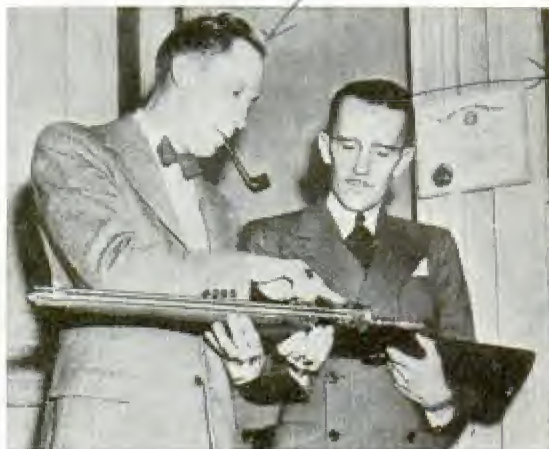
One load of Dry-Ice fires gun about 2,000 times
